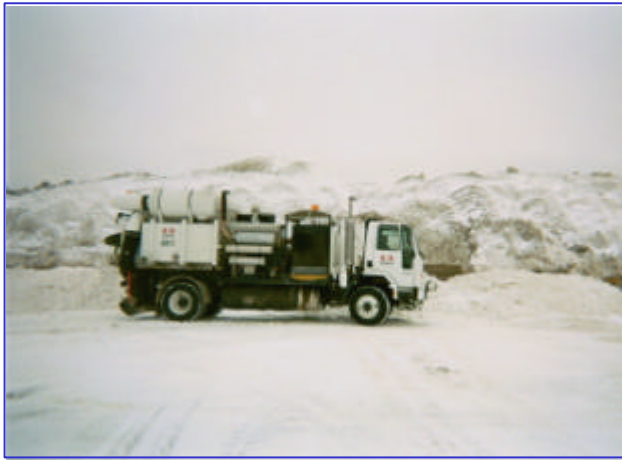
Glycol Recovery Vehicle [GRV] operated by Inland at Buffalo. The GRV is used to remove waste glycol from gate areas following aircraft de-icing.
