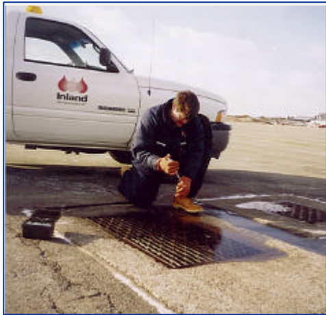
An Inland operator tests fluid at a drain to determine glycol levels present in the fluid and how it will be managed.
