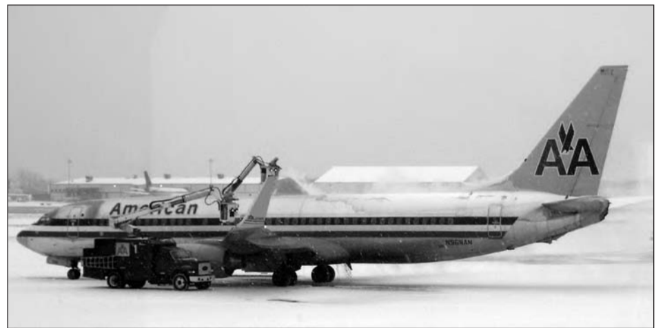
A de-icing operation on February 22, 2008 at Bradley Airport. Aircraft are de-iced as a matter of safety. NASA studies have shown that as little as 0.08 mm of ice on the leading edge of a wing can reduce lift by 25 percent during takeoff.
