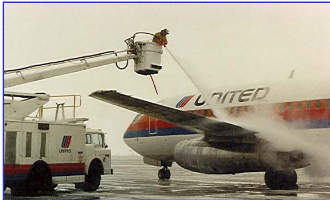
A United Airlines plane is de-iced to remove snow and ice buildup on wing surfaces. United Airlines is using DuraGly P, Inland’s aircraft de-icing fluid made from re-manufactured glycols.
