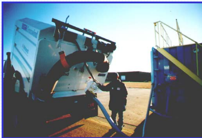
An MGRV at McGuire AFB offloads fluid contaminated with glycol into a temporary storage tank for later recycling.
