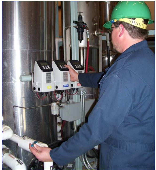
A technician runs a system check on the patented Glycol Concentrator at Inland's Denver airport recycling plant. The units are used to process dilute effluent up to the 50% glycol level.
